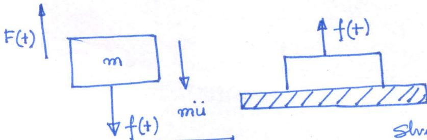
$$\begin{aligned} m\ddot{u} + f(t) &= F(t) \\ s^2 m u(s) + f(s) &= F(s) \end{aligned} \quad (1)$$
