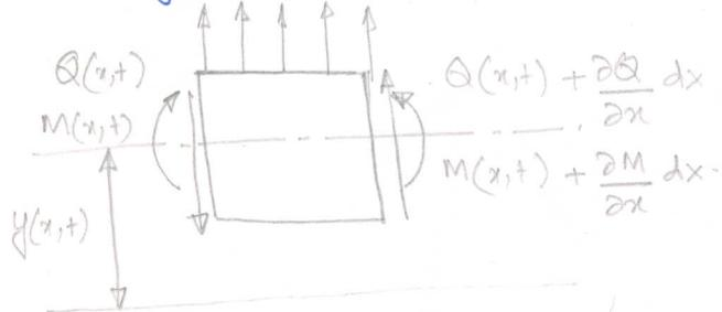
Force balance  $\left[ Q(x,t) + \frac{\partial Q}{\partial x} dx \right] - Q(x,t) + q(x,t) dx = m(x) dx \ddot{y}(x,t)$
