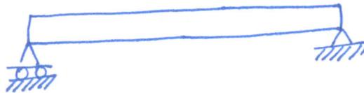
A simply-supported beam is subjected to initial displacement given as,
