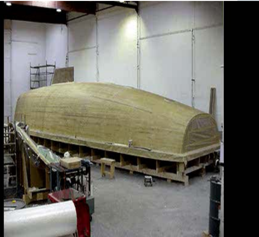
Controlled Vacuum Infusion of the hull of a 64' carbon/epoxy sailing yacht
