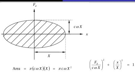
It is of interest to examine the total (elastic & damping) resisting force that is measured in an experiment.
